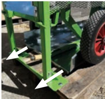
Remove the hopper and the handle arms by passing through the space freed up by the stabilizers, which were raised in the previous step (in the direction indicated by the arrows).
