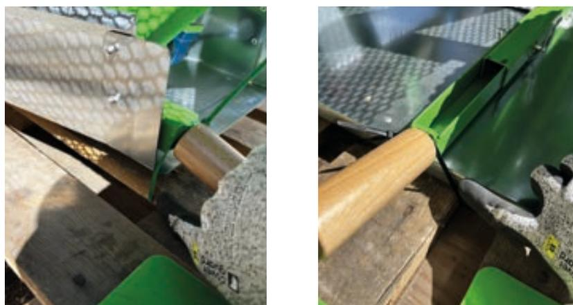
Detach the transport arms and the hopper by cutting the fasteners.
